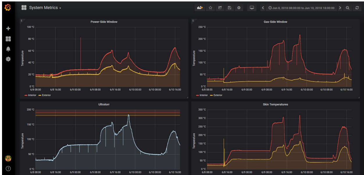
Fig. 22. Grafana dashboard displaying temperature readings. Moving clockwise from the top-left the graphs are displaying: power-side window temperatures, gas-side window temperatures, skin temperatures, and the Ultratorr temperature. Interior is denoted as red while exterior is yellow. The Ultratorr does not a color scheme as it is a single location. Design limitations are set in horizontal yellow lines corresponding to 10 °C from the limit, and horizontal red as the design limitation.
